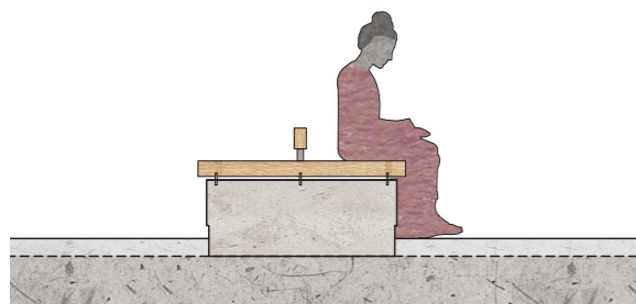
Timber benching on cast plinth
