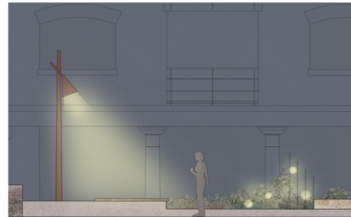
In the long term masts provide high level lighting with atmospheric low level lights integrated in the landscape
